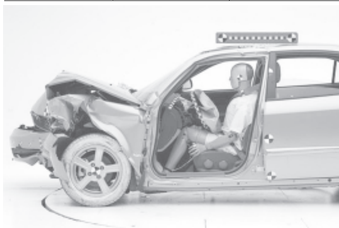
Insurance Institute for Highway Safety photo of a crash test on a 2004 Suzuki Verona. The 2004 Suzuki Verona got a lower safety rating than other inexpensive cars in high-speed crash tests conducted by the insurance industry.—INTERNET
