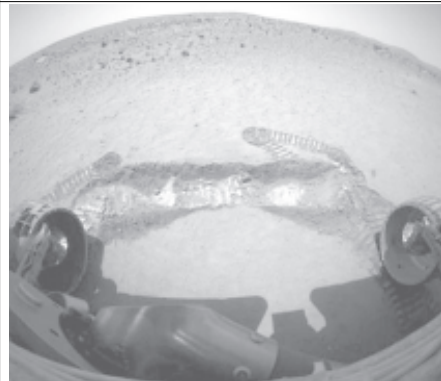
NASA's Mars Spirit rover is shown in front of a 3 inch (7 cm) deep trench created when it dragged its left front wheel back and forth on 20 Feb, 2004. Scientists and engineers will soon begin up-close inspection of the soil in this trench.
