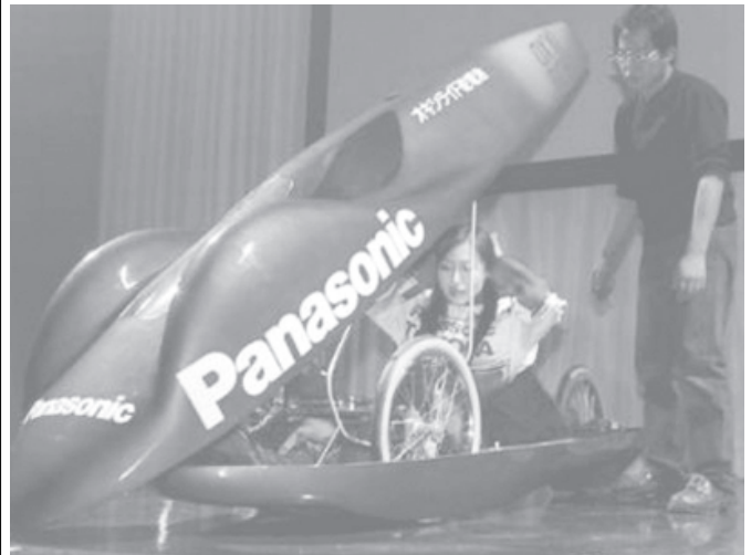
A model gets into a Panasonic luge-shaped vehicle operated by 'Oxyride' dry batteries, developed by Japan's Matsushita Electric Industrial (Panasonic), at an unveiling of the next generation batteries in Tokyo, on 28 Jan 2004. The vehicle can go as far as 1.2 km with two Oxyride AA batteries at a maximum speed of 3.3 km per hour, Matsushita said. The new battery will go on sale in April at 360 yen ($3.40).
