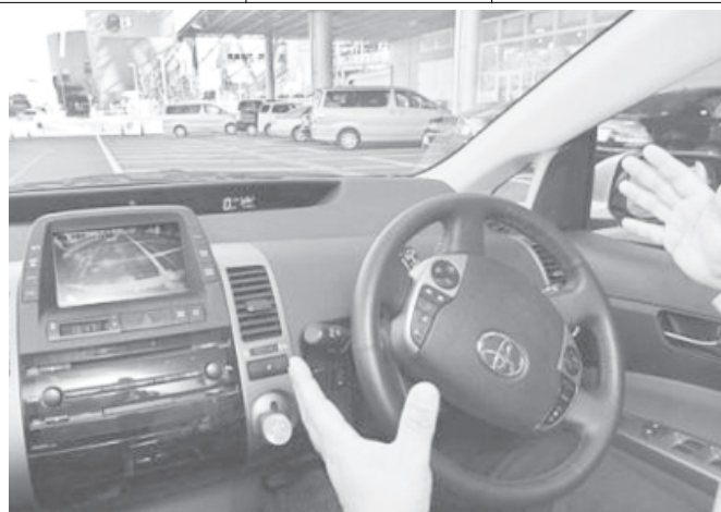
A Toyota employee removes his hands from the steering wheel as the Intelligent Parking system starts backing his car into a narrow parking space during a test drive with The Associated Press in Tokyo on 9 Jan, 2004. Parallel parking is now a breeze for just about anyone with the system that's part of an optional package from Toyota Motor Corp, available only on the Prius hybrid model sold in Japan. — INTERNET
