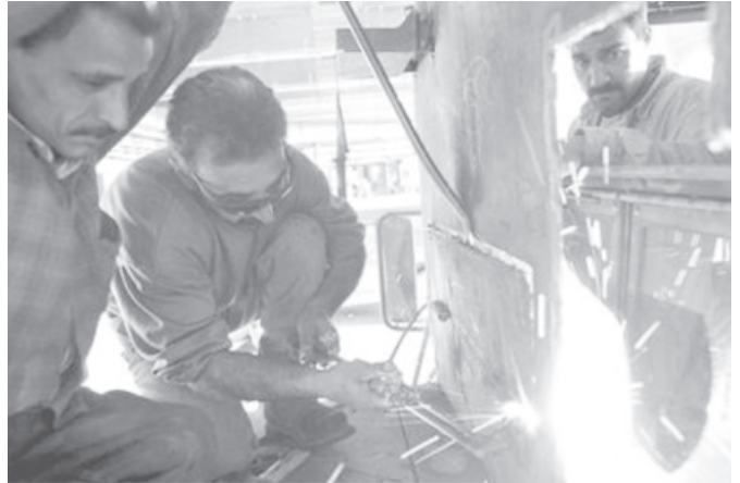
Iraqi civilians contracted by the United States Army, from left, Samir, Adil and Khalil cut a hole in a steel plate that was attached to the front windshield of a 5-ton military truck to shield its passengers from small arms fire and shrapnel on Monday, 29 Dec, 2003 at the Anaconda logistics service area base in Balad, Iraq. With convoys coming under attack by roadside bombs or mortars, transportation units have been forced to add armour and defence weapons to their trucks to shield drivers from injury. —INTERNET
