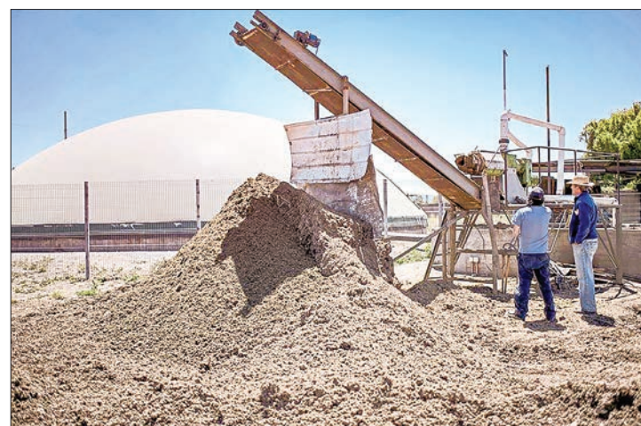
REPRESENTATIONAL PHOTO: The fermentation of pig and cattle manure generates organic fertiliser and biogas (for electricity generation). This biogas plant about 150km south of Santiago, Chile, generates up to 4MW of electricity for the farm's own use. PHOTO: AFP
