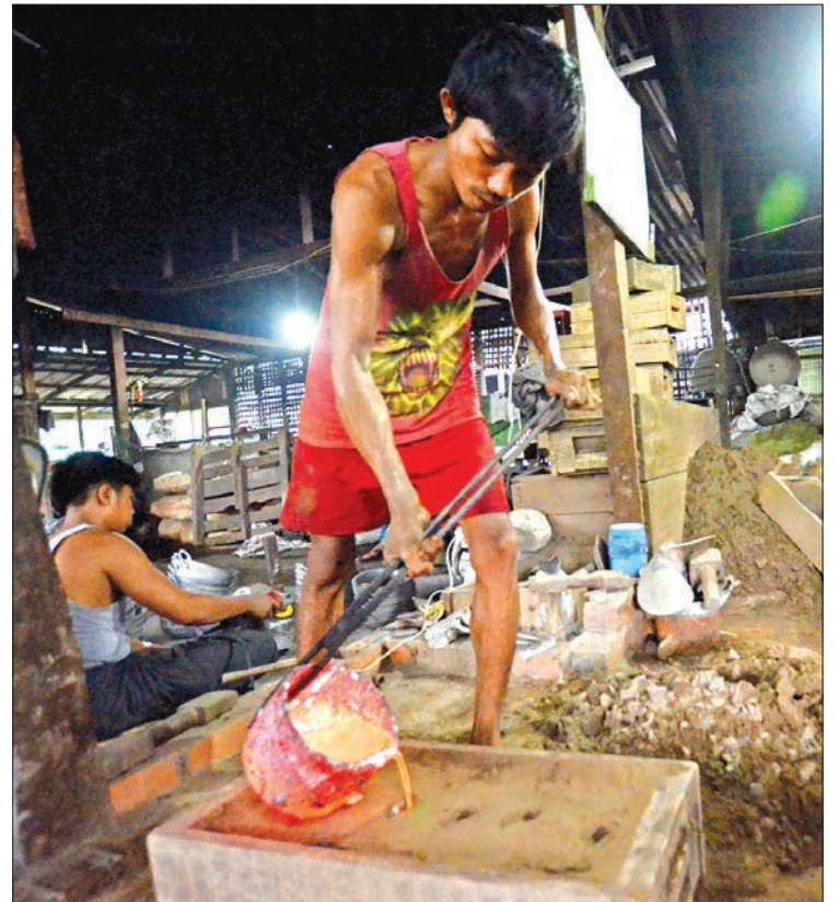
Foundry worker pouring molten metal into casting mold in Kawa Township, Bago Region. PHOTO:PHOE KHWAR
