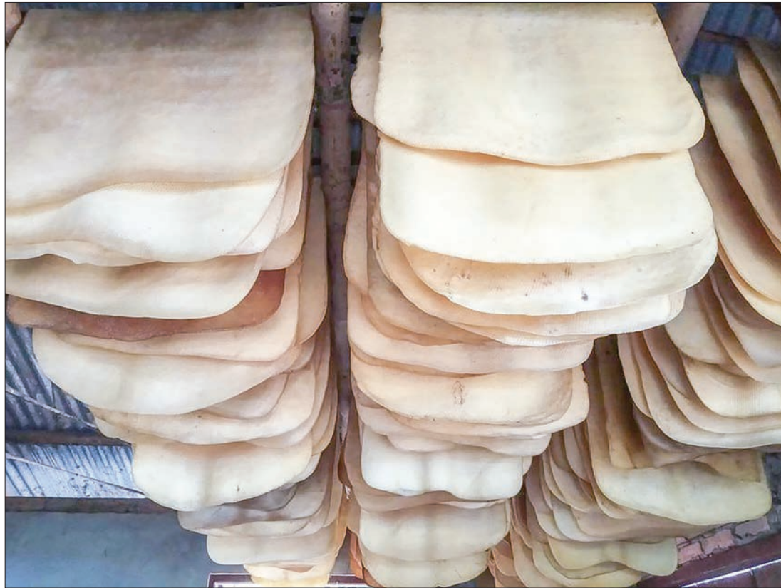
Pressed and rolled latex is smoked and hung up to dry as part of the rubber production process. PHOTO: HTUT HTUT (YE)
