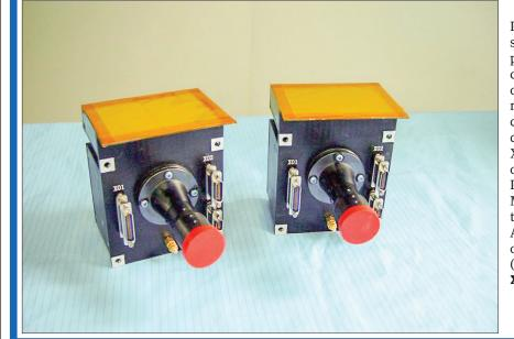
Photo shows samples of the panoramic cameras installed on the lunar rover Yutu-2. The cameras were developed by Xi'an Institute of Optics and Precision Mechanics of the Chinese Academy of Sciences (CAS). PHOTO: XINHUA
