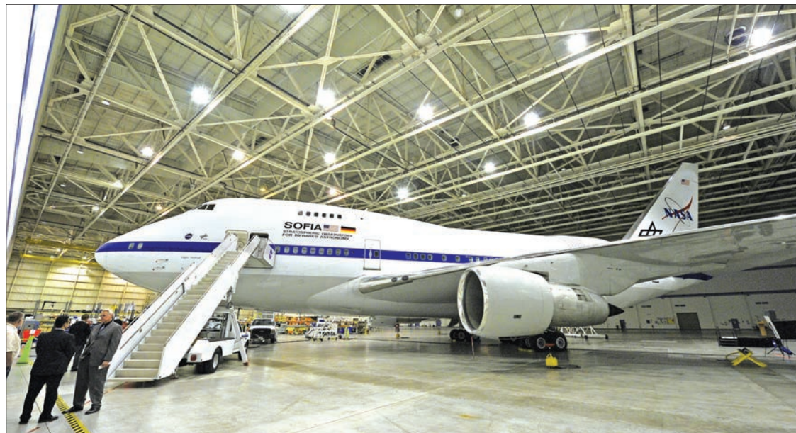
A view of NASA's Stratospheric Observatory for Infrared Astronomy (SOFIA) on 20 April, 2010 on a media preview day at NASA Dryden Flight Research Centre test facility in Palmdale, California. SOFIA, the only flying astronomical observatory in the world, is a specially modified Boeing 747 fitted with a 2.8-metre (98-inch) German-made telescope mounted inside a telescope bay which opens for observation. SOFIA will conduct observation research at altitudes up to 45,000 feet (13,716 metres), getting above more than 99 per cent of the atmospheric water vapour and other infrared-absorbing gases, opening windows to the universe not available from the earth's surface. PHOTO: AFP
