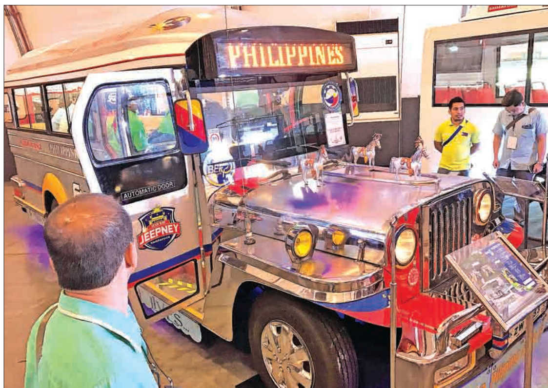
Photo taken on 3 April, 2018 in Manila shows a prototype of a new jeepney which has a door on the side of the vehicle in compliance with the government’s Public Utility Vehicle Modernization Programme. Traditional jeepneys have the door for passengers at the rear. Photo: KYODO NEWS
