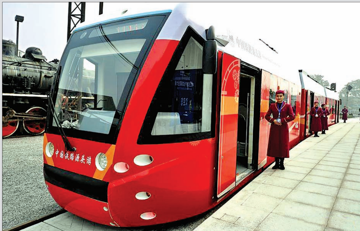
A tram powered by hydrogen fuel cells is seen in Tangshan, north China's Hebei Province on 27 October, 2017. A China-made tram powered by hydrogen fuel cells was put into commercial operation Thursday in Tangshan, north China's Hebei Province. It is the first commercial hydrogen-powered tram in the world and made by China Railway Rolling Corporation (CRR) Tangshan Co, Ltd. PHOTO: XINHUA
